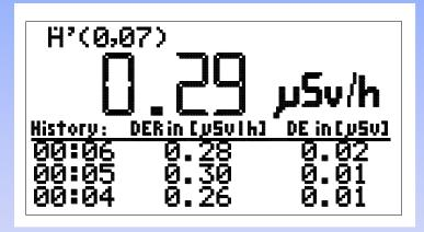
The OD-02 is also capable in dose rate measurement mode
